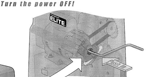
Push the crank tool in hole. Safety releases will separate. Turn the crank to open the gate.
